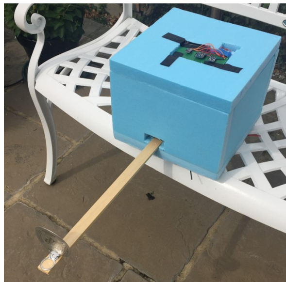
Figure 1: Picture of the payload, highlighting the speed of sound experiment. The ultrasound sensor is point out towards to small metal disc.
